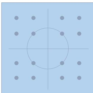
When additional signals are modulated together a higher transfer rate is achieved. In some standards, for example in V.22bis, amplitude and phase modulation are combined (also called QAM **Q**uadrature **A**mplitude **M**odulation), which results in 4 bits being transferred on each modulation.
