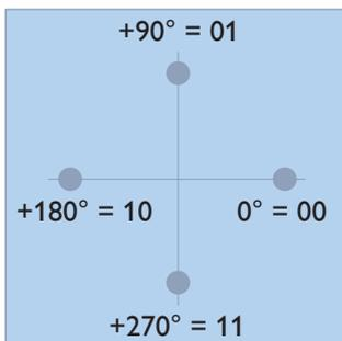
To increase the transfer rate on a telecom modem, more bits are modulated together and transferred via the telephone network. In the adjoining example, the technique of phase modulation is shown where two bits are described by the phase variation of the line signal (V.22).
