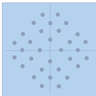
In standards such as V.32, the line is modulated using a technique called TCM (**T**rellis **C**ode **M**odulation), which corresponds to QAM but where a supplement of an extra bit is made for error correction. This is necessary as the border between the transferred bit combinations decreases, which results in a higher error correction requirement.
