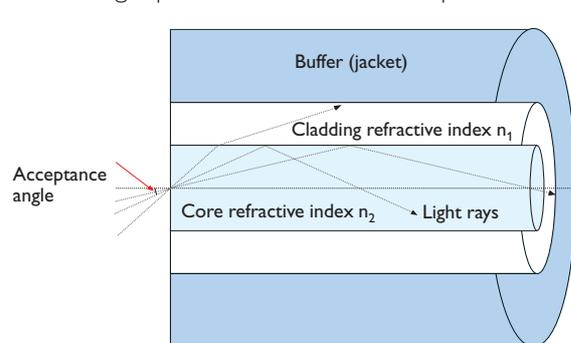
boundary between the two layers act like a mirror provided that the angle of incidence of the light entering the fibre is not too great.
